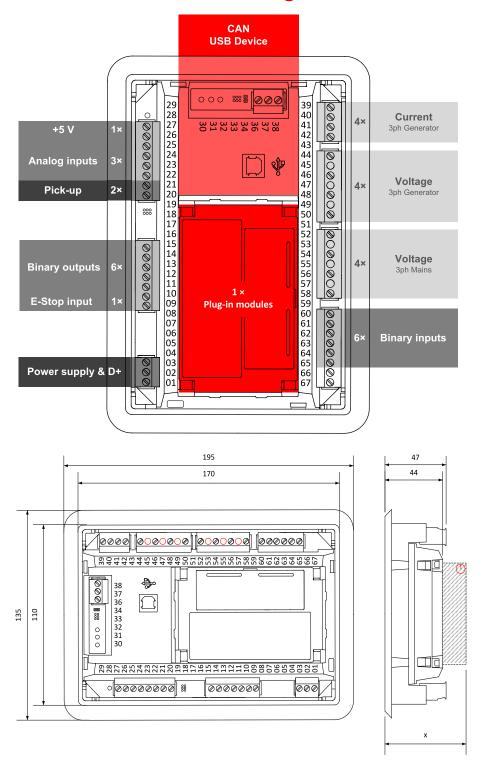
**Note:** The final depth of the controller depends on the selected plug-in module – it can vary between 41 mm and 56 mm. Mind also the size of connectors and cables (e.g. in case of RS232 connector, add about 60 mm more for standard RS232 connector and cable).
