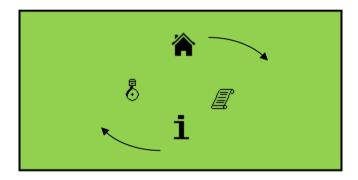
Once the desired icon is at the top, press the **Auto Mode**  $(\checkmark)$  button to enter that instrunmentation section. If the **Auto Mode**  $(\checkmark)$  button is not pressed, the display automatically returns to the Home  $(\ref{alpha})$  page after the configured setting of the *LCD Scroll Timer*.
