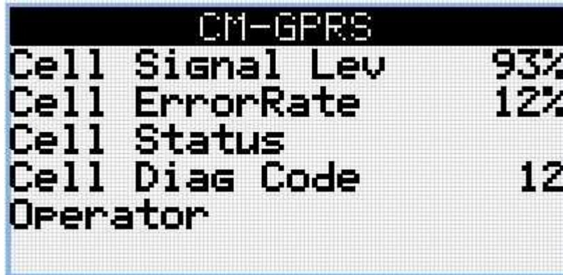
Image 9.18 Main screen of CM-GPRS module
