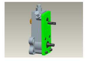
4. The installation rod connection kit(9), and a reset spring set(10).
