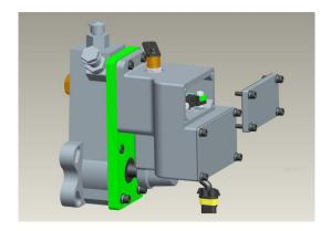
③. The upper chamber of the actuator is communicated with the main oil passage of the oil pump, and the upper cover shall be reliably sealed to prevent oil leakage. The status of the actuator after installation is shown as Fig.:
