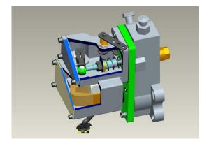
The position of the arm and the bearing is adjusted according to the structure size of different injection pumps when leaving the factory, and the user generally does not need to adjust. Under special circumstances, the O oil supply does not match, the user can make appropriate adjustments.
